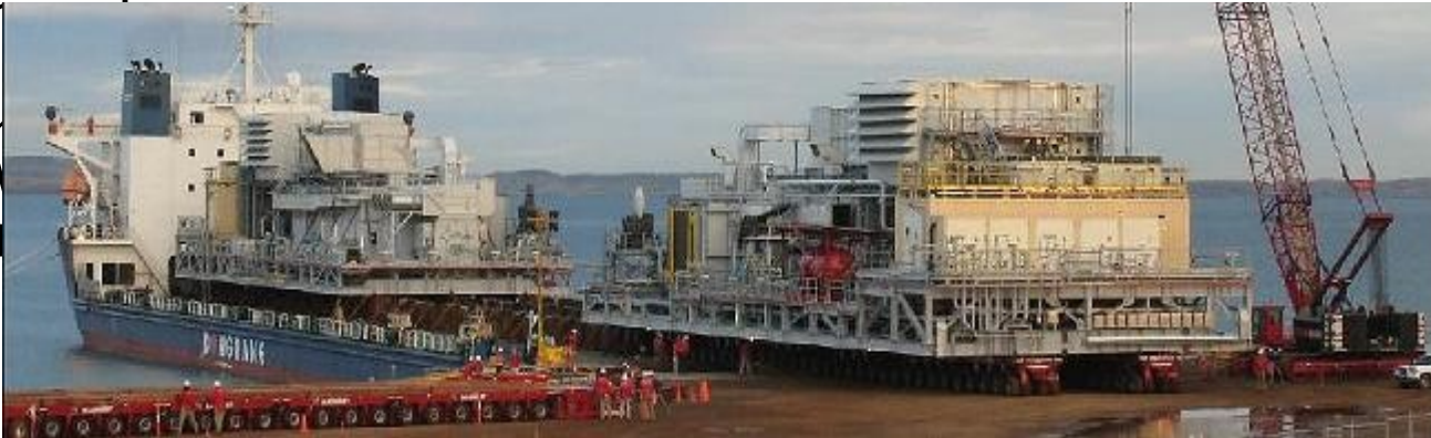
Pluto Project large LNG modules being unloaded at Burrup Peninsula Site from special “low loader vessel”
